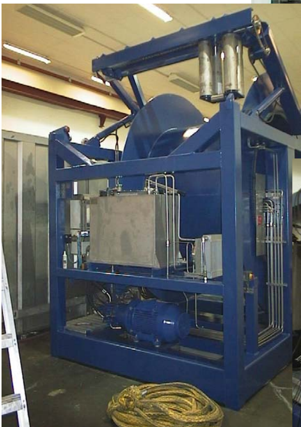
Built on zone 2 rated hydraulic power unit.
